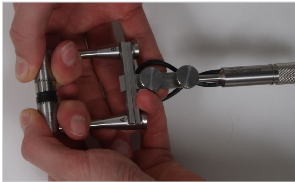
Figure 19.6 - Loosen the spacer adjustment knob and pull the microphones apart carefully.
