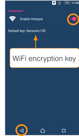
Figure 19.12 - Switch on the Hotspot, note the encryption key and accept with the back button.
