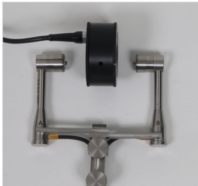
Figure 19.19 - Dismantle the probe, spacer and sleeve.
