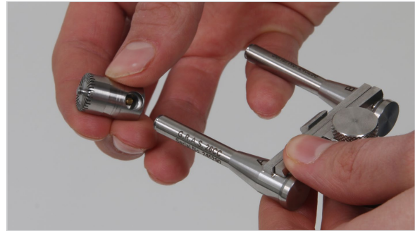
Figure 19.2 - Mount the microphone and adapter on to the preamplifier.
