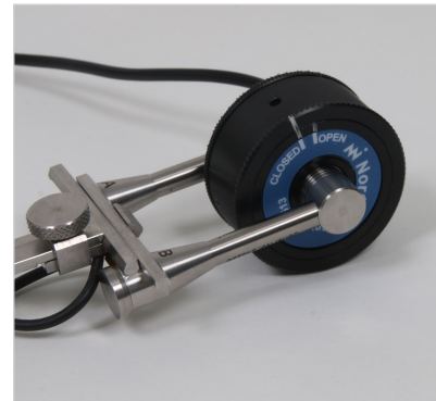
Figure 19.21 - Tighten the spacer and knob, and close the Nor1294.
